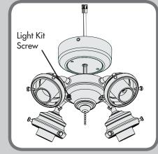
Feed the light kit wires through the center hole in the switch housing. Then attach the switch housing to the light kit by installing the light kit screws into the bottom of the switch housing.
