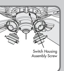
Lift the light kit up to meet the upper switch housing. Install the switch housing assembly screws. Tighten screws.
