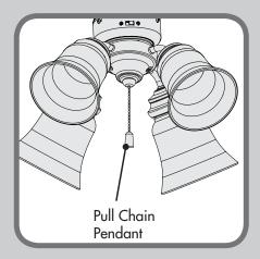
To turn lights on and off, pull the pull chain pendant coming from the center of the light kit.
