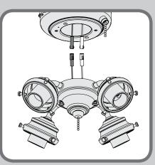
Using the single pin connectors, connect the black or blue wire from the fan to the black wire from the light kit. Connect the white wire from the fan to the white wire from the light kit. Note: Do not allow the light kit to hang only
