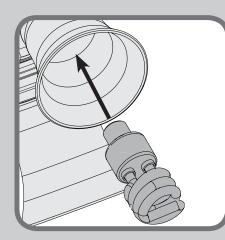
Installing the bulb - Install a bulb into each socket. When necessary, replace bulbs with bulbs of same type and wattage.
