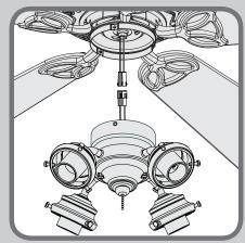
Using the single pin connectors, connect the black or blue wire from the fan to the black wire from the light kit. Connect the white wire from the fan to the white wire from the light kit. Note: Do not allow the light kit to hang only by the wire connectors.
