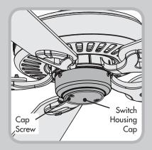
If your fan's switch housing cap resembles this one, remove the cap screws with a Phillips head screwdriver. Then follow the instructions for **TYPE-A ASSEMBLY.**  If your fan's switch housing cap resembles this one, remove the whole switch housing by removing the switch housing screws with a Phillips head screwdriver. Remove the plug button. Then follow the **TYPE-B ASSEMBLY INSTRUCTIONS.**
