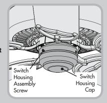
If your fan's switch housing cap resembles this one, remove the whole switch housing by removing the switch housing screws with a Phillips head screwdriver. Remove the two cap screws from the inside of the switch housing. Reinstall the switch housing. Tighten the switch housing screws. Then follow the instructions for **TYPE-A ASSEMBLY**.
