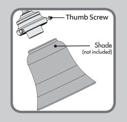
Installing the shades - To install the shade, first loosen the thumb screws. Raise the shade to the light fixture. Tighten all thumbscrews securely.
