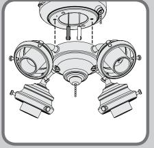
Lift the light kit up to meet the lower switch housing. Guide the two pre-installed light kit screws into the holes in the lower switch housing. Tighten screws.
