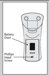
To access the battery compartment, remove the small Phillips head screw that secures the battery door to the transmitter assembly. The battery should be installed with the positive (+) side up. Replace with a CR2032 battery when necessary.
