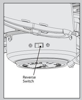
To switch the direction of air flow, move the reverse switch to the opposite position. You will need to remove the light kit glass to do so.
