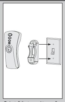
To install the transmitter cradle, remove the two screws holding your switch cover plate. Do not remove the cover plate. Orient the cradle by lining up the two mounting holes with those on the cover plate. Insert and tighten the screws. Do not over tighten.
