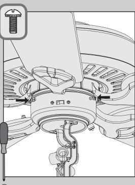
Install the third switch housing screw.
