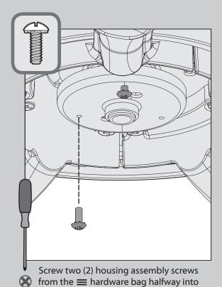
the motor housing. It does not matter
