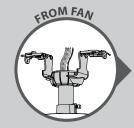
Using an orange wire connector from the ★ hardware bag, connect the 3 grounding wires (green, green/yellow stripe, or bare copper) coming from the ceiling, downrod, and
