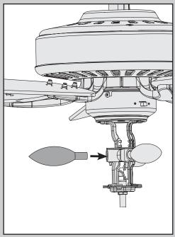
Install a light bulb in each socket.
