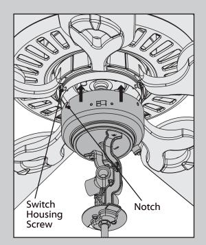
Align the notches in the sides of the lower switch housing with the upper switch housing screws. Lift the lower switch housing. Twist the lower switch housing clockwise to lock into place.
