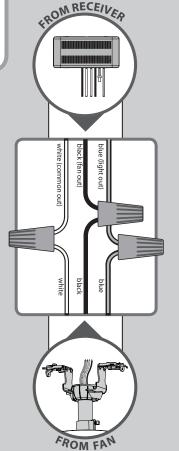
Using an orange wire connector from the hardware bag, connect the black wire (ungrounded) from the ceiling to the black wire from the receiver (marked "live in"). Connect the white wire (grounded) from the ceiling to the white wire from the receiver (marked "neutral in").
