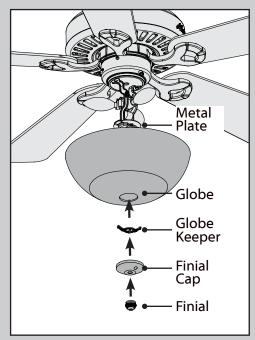
Press the globe and globe keeper flush against the metal plate.
