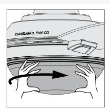
Attach the globe by lifting and turning clockwise a quarter of a full turn or the glass until it stops.
