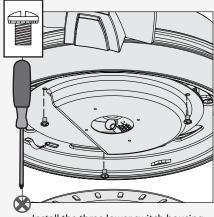
Install the three lower switch housing screws, found in the == hardware bag, into place and then tighten all three screws securely.
