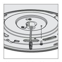
Feed the 9-pin wire plug through the center hole of the upper switch housing, then wrap keyhole slots around the screws and twist counterclockwise. Insert the third upper switch housing screw, found in the hardware bag, into place and then tighten all three screws.
