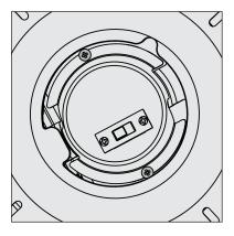
Remove the switch housing cap by removing the two light kit assembly screws.
