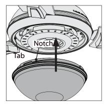
Lift the globe and align the notches in the globe with the tabs in the light kit.
