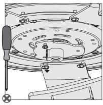
Remove the remaining two screws...
