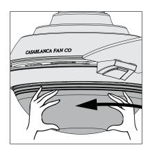
Remove the globe by lifting and turning counterclockwise one third of a full turn of the glass. Cautiously lower the glass and set aside.
