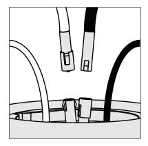
Slide the switch housing cap through the hole in the center of the LED assembly. Remove the dummy terminals from the blue and white pin connectors in the switch housing. Connect the pin connectors from the switch housing and the LED assembly.
