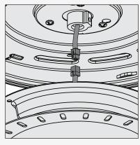
Connect the plugs from the upper and lower switch housings. Make sure to line up the colored markings on the connectors.
