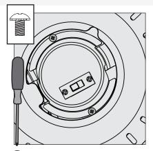
Attach the switch housing cap to the lower switch housing by installing two light kit assembly screws, found in the hardware bag.
