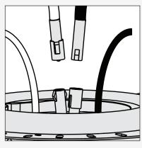
Disonnect the pin connectors from the switch housing and the LED assembly. Set aside the components.
