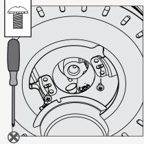
Attach the LED assembly to the switch housing by installing two light kit assembly screws, found in the hardware bag, through the slots, not the screw holes.
