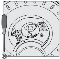
Remove the LED assembly by removing the two light kit assembly screws. Set aside the components.
