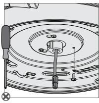
Remove the screw from the non-keyholed slot. Rotate the switchhousing clockwise and remove. Set aside the components.
