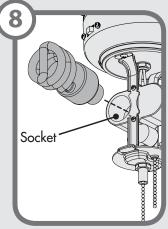
Installing the bulb - Install a bulb into each socket. When necessary, replace bulbs with bulbs of same type and wattage.
