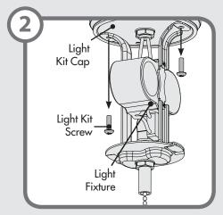
Remove the screws attaching the light kit cap to the light fixture. Discard the screws.
