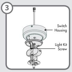
Feed the light kit wires through the center hole in the switch housing. Then attach the switch housing to the light kit by installing the light kit screws into the bottom of the switch housing.
