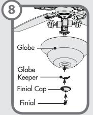
Installing the globe - Press the globe and globe keeper flush against the metal plate. Thread the light pull chain through the hole in the center of the finial cap and thread the fan pull chain through the hole in the side of the cap. Finally, thread only the light pull chain through the hole in the finial and screw the finial onto the threaded rod.
