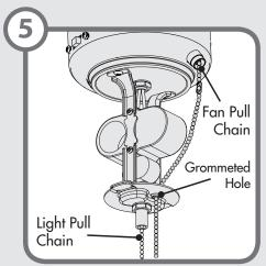
If necessary, attach the extension chain provided to the fan pull chain coming from the switch housing. Then feed the end of the extension chain through the grommeted hole in the light kit.
