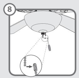
Installing the Pull chain pendant -Attach the pull chain pendants to the end of the short chains coming from the switch housing and the light kit. Turn on power. Your installation is complete!
