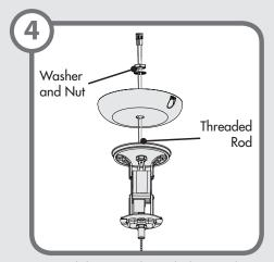
Feed the wires through the switch housing cap, washer, and nut. Then install the switch housing cap by twisting clockwise onto the threaded rod. Install the washer and nut onto threaded rod and tighten securely.
