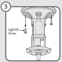
Remove the light kit screws attaching the light kit cap to the light fixture.
