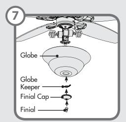
Installing the globe - Press the globe and globe keeper flush against the metal plate. Thread the light pull chain through the hole in the center of the finial cap and thread the fan pull chain through the hole in the side of the cap. Finally, thread only the light pull chain through the hole in the finial and screw the finial onto the threaded rod.
