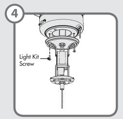
Attach the light kit to the switch housing by re-installing the light kit screws through the fixture and light kit cap into the switch housing.
