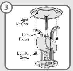
Install the shorter light kit screws, found in the hardware bag, through the light fixture and into the light kit cap.
