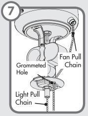
If necessary, attach the extension chain provided to the fan pull chain coming from the switch housing. Then feed the end of the extension chain through the grommeted hole in the light kit.
