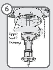
Lift the light kit assembly up so that the screw holes in the lower switch housing line up with the holes in the upper switch housing. Install the switch housing screws and tighten securely.
