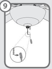
Installing the pull chain pendant - Attach the pull chain pendants to the end of the short chains coming from the switch housing and the light kit. Turn power on. Your installation is complete.
