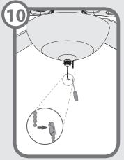
Installing the pull chain pendant - Attach the pull chain pendants to the end of the short chains coming from the switch housing and the light kit. Turn power on. Your installation is complete.
