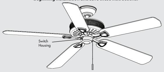
Your light kit is compatible with most ceiling fans. The light kit will attach to the fan's switch housing. Begin on page 3 where you will choose the type of switch housing that most closely resembles the one on your fan. From there, you will be directed to the set of assembly instructions that are appropriate for installing the light kit to your fan.
