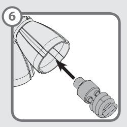
Installing the bulb - Install a bulb into each socket. When necessary, replace bulbs with bulbs of same type and wattage.
