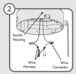
Using the provided wire connectors connect the white wire from the fan to the white wire from the wire harness and connect the black or blue wire from the fan to the black wire from the wire harness.
