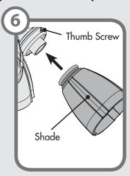
Installing the shade - First loosen the thumb screws. Raise the shade to the light fixture. Tighten all thumbscrews securely.
