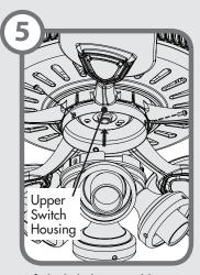
Lift the light kit assembly up so that the screw holes in the lower switch housing line up with the holes in the upper switch housing. Install the switch housing screws and tighten securely.
