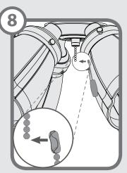
Installing the pull chain pendant - Attach the pull chain pendant to the end of the short chains coming from the switch housing and the light kit.
