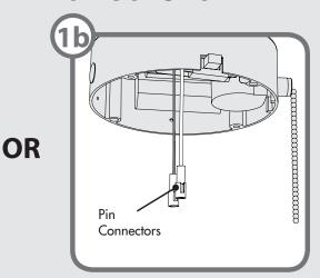
If the fan has pin connectors, cut the wires just above the fan pin connectors with wire cutters. Discard the pin connectors. Go to step 2.
