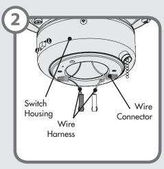
If your fan does not have pin connectors on the wires coming from the switch housing, install the wiring harness provided. Using the provided wire connectors connect the white wire from the fan to the white wire from the wire harness and connect the black or blue wire from the fan to the black wire from the wire harness.
