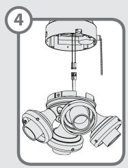
Using the single pin connectors, connect the black or blue wire from the fan to the black wire from the light kit. Connect the white wire from the fan to the white wire from the light kit.
