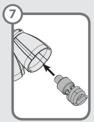
Installing the bulb - Install a bulb into each socket. When necessary, replace bulbs with bulbs of same type and wattage.
