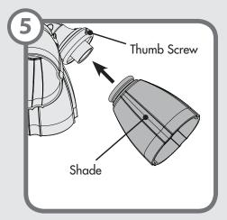
**Installing the shade** - First loosen the thumb screws. Raise the shade to the light fixture. Tighten all thumbscrews securely.
