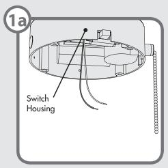
If your fan does not have pin connectors on the wires coming from the switch housing, go to step 2.
