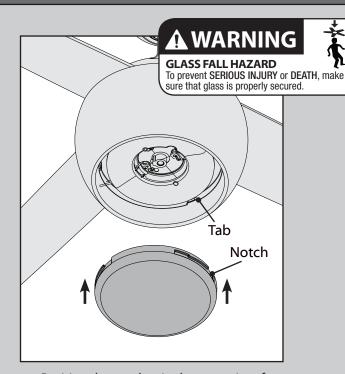
Position the notches in the outer rim of the globe so they line up with the three tabs on the inside rim of the housing. Carefully lift the globe up inside the housing as far as it will go, then rotate the globe clockwise until it is held tightly in place by the tabs.
