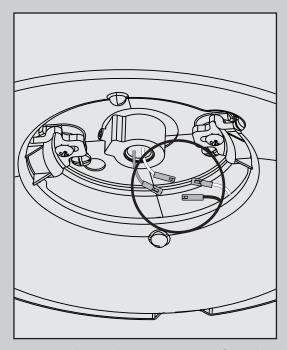
Connect the single-pin connectors from the LED assembly to the connectors from the fan. Connect the white wires together. Connect the blue and black wires together. Tuck the excess wiring above the LED assembly.
