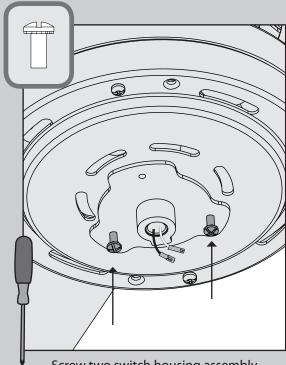
Screw two switch housing assembly screws, found in the ≡ hardware bag, halfway into the mounting plate on the bottom of the motor housing. It does not matter which two screw holes you choose.
