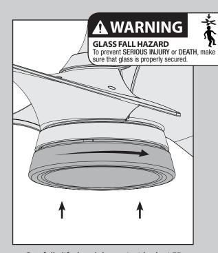
Carefully lift the globe up inside the LED assembly as far as it will go, then rotate the globe clockwise until it is held tightly in place by the tabs.
