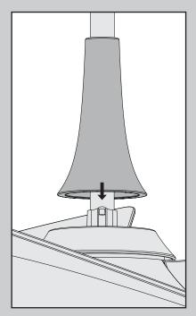
Lower the adapter cover until it rests on top of the motor housing.
