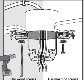
(included) when securing to support structure with approved electrical outlet box. Drill 9/64" pilot holes in support structure to aid in securing ceiling bracket with hardware found in the \*\psi\$ hardware bag.
