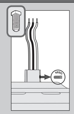
Remove the pre-installed setscrew so that the downrod can be inserted.
