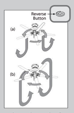
The reverse button on the wall control changes the air flow pattern. In warm weather, use (a) downward air flow pattern. In cold weather, use (b) upward air flow pattern.
