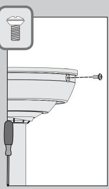
Install the two canopy screws found in the hardware bag.
