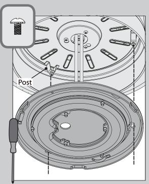
Screw two LED assembly screws, found in the = hardware bag. halfway into two of the posts in the upper switch housing. Push any excess wiring into the switch housing, then wrap the keyhole slots in the LED assembly around the screws and twist clockwise.
