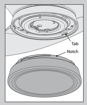
Position the notches in the outer rim of the globe so they line up with the three tabs on the inside rim of the LED assembly.
