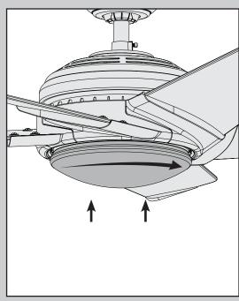
Carefully lift the globe up inside the light kit as far as it will go, then rotate the globe clockwise until it is held tightly in place by the four tabs.
