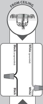
Using orange wire connectors from the hardware bag, connect the black wire (ungrounded) from the ceiling to the black wire from the fan.
