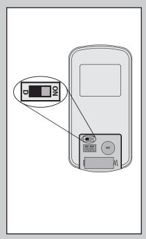
If a light kit is installed on your fan, choose the light bulb mode by moving the toggle switch. For LED light kits, set the switch to "ON." Replace the battery door.
