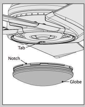
Position the notches in the outer rim of the globe so they line up with the tabs on the inside of the rim on the light kit.
