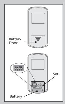
Remove battery door. Change the dip switch settings if the frequency matches a previously installed remote transmitter. Install A23 or MN21 alkaline battery in the proper polarity and replace the battery door. To pair the remote, hold down the Set button for 5 seconds. Pairing is complete when the small LED button on the remote flashes twice.
