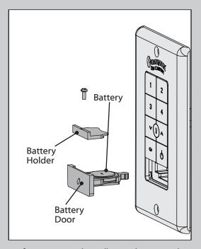
Before operating the wall control, press on the battery door to eject it. Unscrew the battery holder. Insert the battery, found in the control hardware bag, with the positive (+) side facing downward. Reinstall the battery holder and reinsert the battery door into the wall control.
