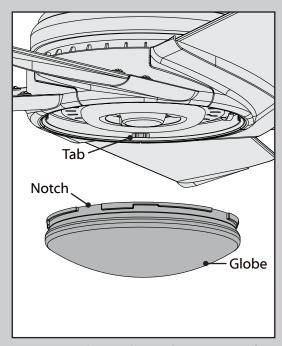
Position the notches in the outer rim of the globe so they line up with the tabs on the inside of the rim on the light kit.
