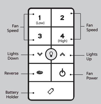
Quickly press the up or down arrow to turn the lights off and on. Hold the up or down arrow to raise or dim the light level. The reverse button changes the direction that the blades turn. The power button turns the fan off and on.
