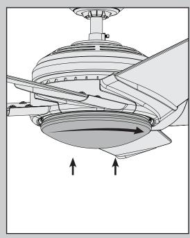
Carefully lift the globe up inside the light kit as far as it will go, then rotate the globe clockwise until it is held tightly in place by the four tabs.
