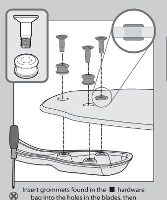
bag into the holes in the blades, then secure each blade to a blade iron with screws found in the  $\blacktriangle$  hardware bag.
