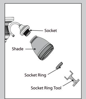
Remove the socket rings from the sockets. Install the shades onto the sockets. Install the socket rings onto the sockets. Tighten them by turning clockwise with the socket ring glass tool.
