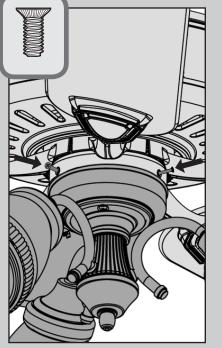
Install the three switch housing screws, found in the ≡ hardware bag.
