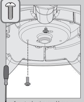
Screw two housing assembly screws
