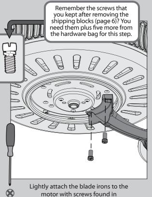
the X hardware bag, then securely tighten after both screws are attached.
