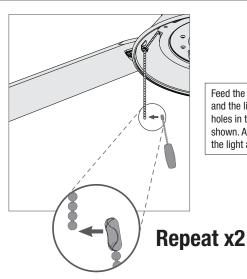
Feed the pull chains from the fan switch and the light switch down through the holes in the upper switch housing as shown. Attach the pull chain pendants to the light and fan pull chains.
