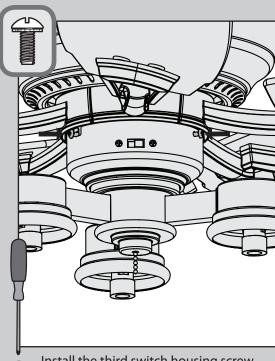
Install the third switch housing screw.
