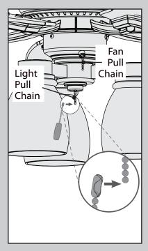
Remove and discard the plastic connectors from the ends of the pull chains (if necessary), then connect the appropriate pull chain pendant to each of the short chains coming from the switch housing.
