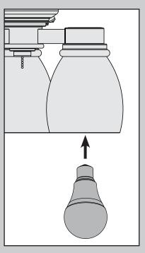
Install a light bulb in each socket.
