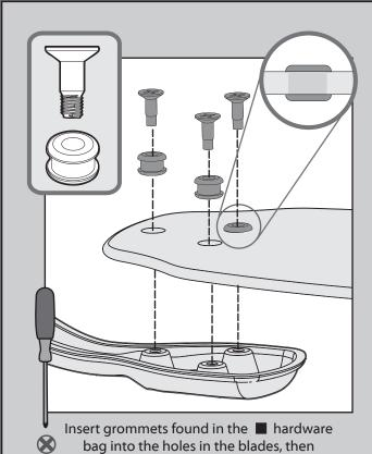
secure each blade to a blade iron with screws found in the **A** hardware bag.
