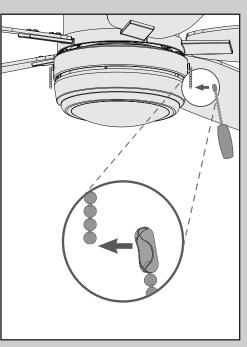
Connect the appropriate pull chain pendant to each of the short chains. The fan pull chain controls the speed: from high to off. The light pull chain controls the light fixture: on and off.
