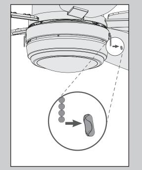
Remove and discard the plastic connectors from the ends of the short pull chains coming from the sides of the light kit assembly.
