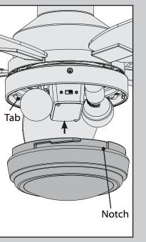
Align the notches in the outer rim of the globe with the tabs on the light kit assembly. Carefully lift the globe up inside the light fixture as far as it will go. Rotate the globe in a clockwise direction until it is held tightly in place by the three tabs.
