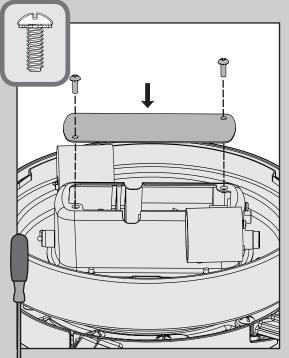
Carefully push all switch housing components into the switch housing, then install the switch housing plate using two light kit assembly screws, found in the ≡ hardware bag.
