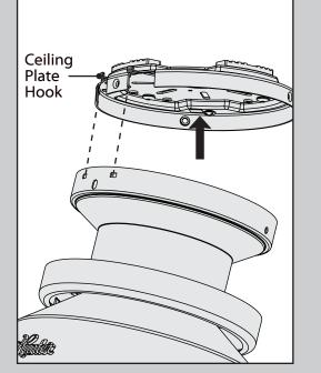
Raise the fan and align the slots in the canopy with the hooks on the ceiling plate. **Note:** To hang the fan, you must tilt the canopy to an almost vertical position so that the canopy slots sit on the ceiling plate hooks.
