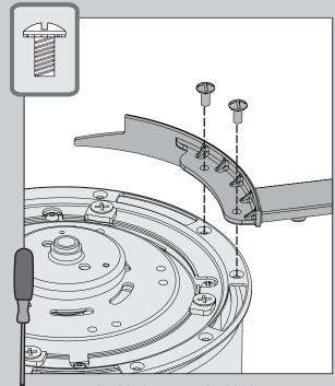
Install a blade iron to the blade iron mounting plate using two blade iron assembly screws, found in the X hardware bag. Repeat this process to install all five blade irons.
