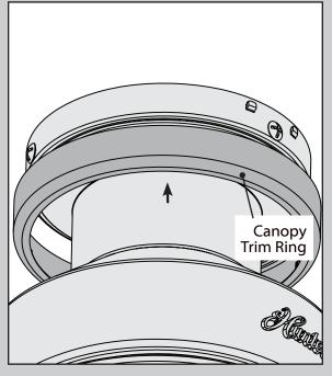
Using both hands, push the canopy trim ring up to the top of the canopy. The canopy trim ring will snap and lock into place.
