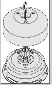
Thread the wires through the top housing.
