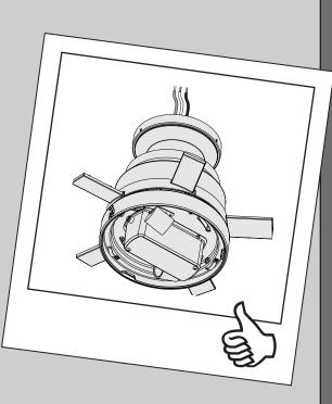
Make sure the light kit assembly is securely attached to the motor housing. Failure to properly secure all three assembly screws could result in the light fixture falling.
