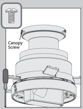
Hold the canopy up with the screw holes aligned. Partially install two canopy screws, found in the hardware bag, into the holes opposite the ceiling plate hooks.
