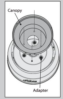
Place the canopy on the top housing. Ensure all four screw holes line up with the screw holes in both the top housing and the adapter.
