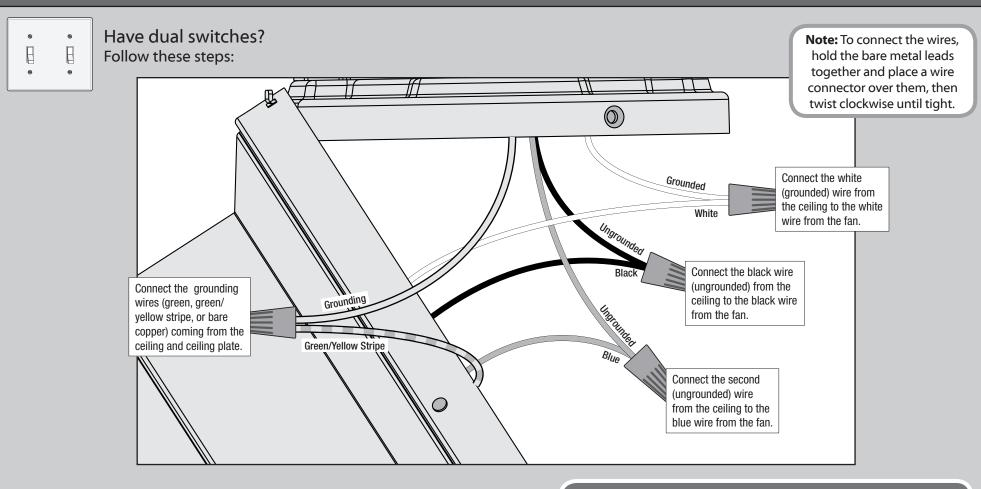
Turn the splices upward and push them carefully back through the hanger bracket into the outlet box. Spread the wires apart, with the grounded wires on one side of the outlet box and the ungrounded wires on the other side of the outlet box.
