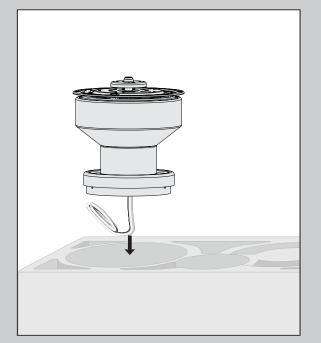
Carefully turn the motor assembly upside down and place it in one of the holes in the packaging.
