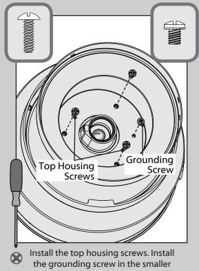
screw hole. These screws can be found in the hardware bag.
