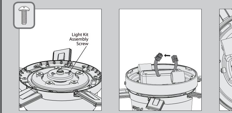
Partially install two light kit assembly screws, found in the ≡ hardware bag, halfway into the motor housing as shown. It does not matter which two screw holes you choose. Feed the 9-pin plug connector coming from the bottom of the motor housing through the center hole in the light kit assembly. Connect it to the plug connector found in the switch housing area of the light kit assembly. Make sure to line up the colored markings on the connectors.
