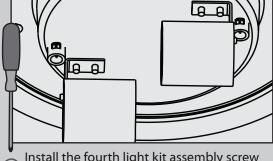
Install the fourth light kit assembly screw and tighten all four screws securely.
