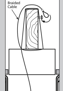
Wrap the braided cable around the support brace once creating a complete circle. Hook the looped end of the cable over the wood screw so that the cable lies between the washer and the support brace.
