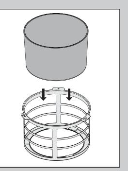
Carefully lower the globe into the globe retainer until it rests in place.
