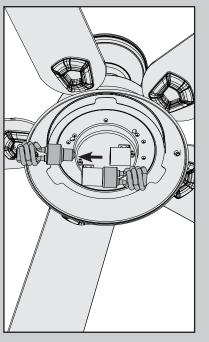
**Changing the bulbs** - carefully remove the globe assembly. Unscrew the bulbs and replace with bulbs of the same wattage. Reinstall the globe assembly.
