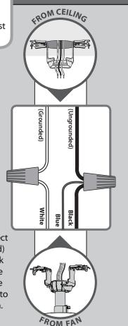
For Dual Switches Using the orange wire connectors from the ★ hardware bag, connect the white wire (grounded) from the ceiling to the white wire from the fan.
