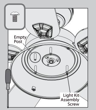
Partially install three light kit assembly screws, found in the = hardware bag, into the posts as shown, leaving the circled post empty.
