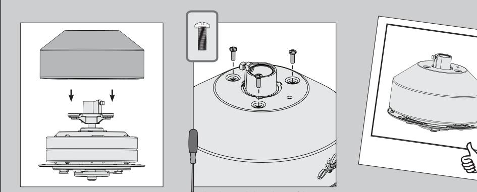
Gently lower the motor housing so it rests in place on the motor assembly.
