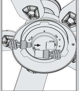
Install a bulb into each of the sockets. When necessary, replace with bulbs of the same wattage.
