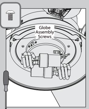
Partially install two globe assembly screws, found in the ≡ hardware bag, halfway into the light kit assembly as shown. It does not matter which two screw holes you choose.
