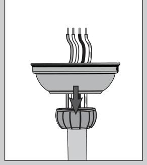
Put the wires and downrod through the canopy. Let the canopy sit loosely on top of the fan.
