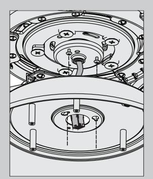
Feed the wire plug through the center hole of the upper switch housing, then wrap keyhole slots around the two screws and twist counterclockwise to lock the upper switch housing into place.
