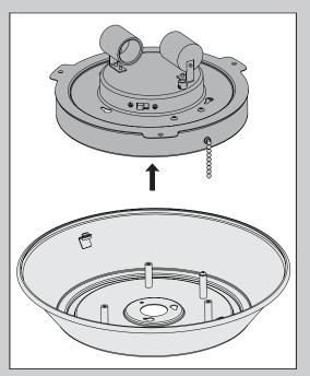
Carefully remove the light kit from the upper switch housing and set the light kit aside.
