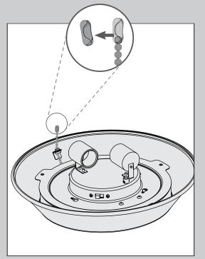
Remove and discard the plastic connectors from the ends of the two pull chains.
