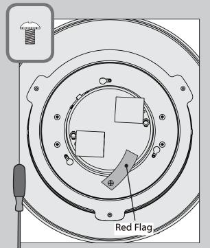
Remove the pre-installed light kit assembly screw and red flag from the light kit assembly. **Save the screw. It will be needed for light kit installation.**
