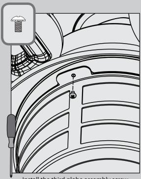
Install the third globe assembly screw and tighten all three screws securely.
