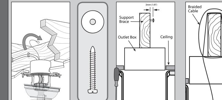
Insert the looped end of the braided cable through the ceiling bracket and one of the holes in the outlet box into the ceiling. Access the support brace in the ceiling. You may not be able to do this from below the ceiling depending on your installation site.
