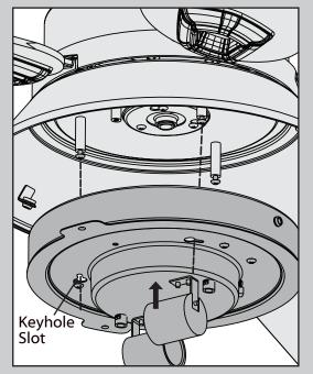
Align the three keyhole slots in the light kit with the three assembly screws in the posts. Lift the light kit and twist clockwise to lock it into place. Be sure that both pull chains are hanging freely.
