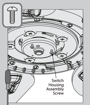
Partially install two switch housing assembly screws ,found in the ≡ hardware bag, into the motor housing as shown. It does not matter which two screw holes you choose.
