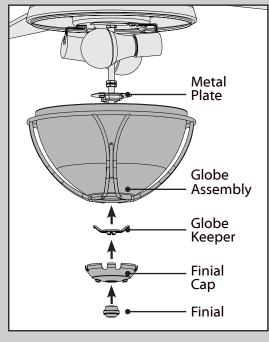
Press the globe assembly and globe keeper flush against the metal plate. Make sure the cage fits into place inside the upper switch housing. Thread the pull chains through the holes in the finial cap, then screw the finial onto the threaded rod.
