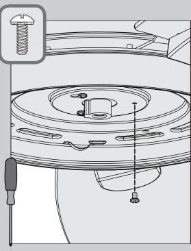
Insert the third screw, found in the ≡ hardware bag, into place and tighten all three screws securely.
