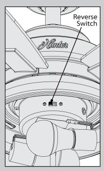
changing the direction of air flow unscrew the finial and remove it from the threaded rod. Remove the finial cap and unscrew the globe keeper while supporting the globe assembly with your other hand. Carefully remove the globe assembly. Move the reverse switch to the opposite position.
