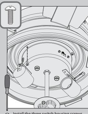
Install the three switch housing screws found in the ≡ hardware bag.
