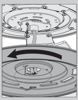
Feed the 9-pin wire plug through the center hole of the upper switch housing, then wrap keyhole slots around the screws and twist counterclockwise.
