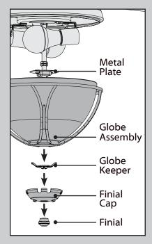
Changing the bulbs - unscrew the finial and remove it from the threaded rod. Remove the finial cap and unscrew the globe keeper while supporting the globe assembly with your other hand. Carefully remove the globe assembly. Unscrew bulbs and replace with bulbs of same type and wattage. Reinstall the globe assembly.
