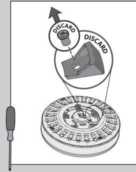
Remove the shipping blocks from the motor. Discard the screws.
