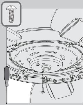
Screw two switch housing assembly screws from the = hardware bag halfway into the motor housing. It does not matter which two screw holes you choose.
