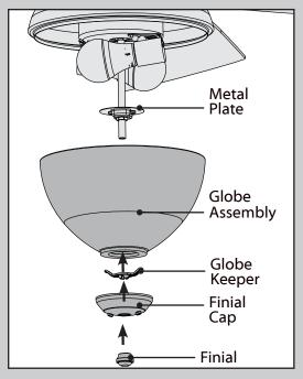
Press the globe assembly and globe keeper flush against the metal plate.
