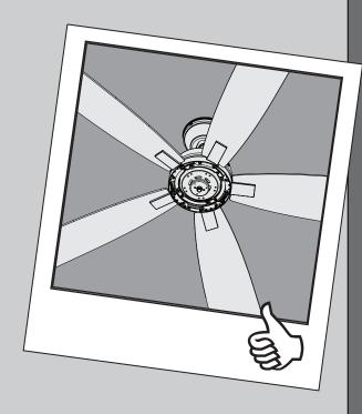
Lightly attach the blade irons to the motor housing with screws found in the X hardware bag, then securely tighten after both screws are attached.
