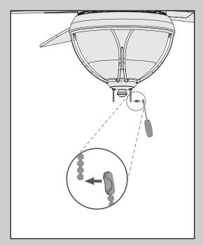
Connect the appropriate pull chain pendant to each of the short chains coming from the finial cap. The fan pull chain controls the speed: from high to off. The light pull chain controls the light fixture: on and off.
