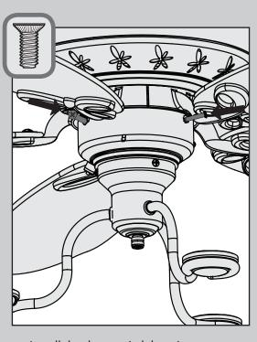
Install the three switch housing screws found in the  $\equiv$  hardware bag.
