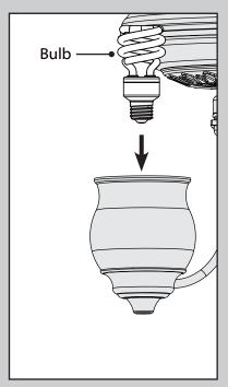
Install a bulb into each of the sockets. When necessary, replace with bulbs of same wattage.
