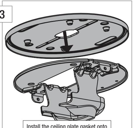
Install the ceiling plate gasket onto the ceiling plate. The four holes in the ceiling plate should lineup with the four posts in the gasket.
