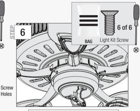
Install the three switch housing screws found in the **=** hardware bag
