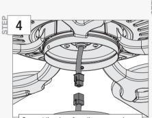
Connect the plugs from the upper and lower switch housings. Make sure to line up the colored markings on the connectors.
