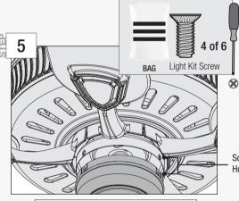
Lift the lower switch housing up until its screw holes are aligned with the screw holes in the upper switch housing.
