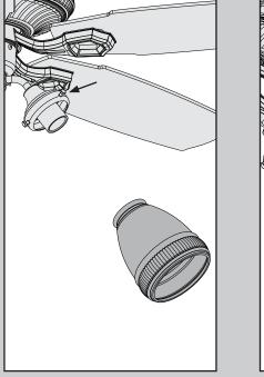
To install the shade, first loosen the thumb screws. Raise the shade to the light fixture. Tighten all thumbscrews securely.
