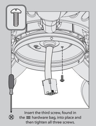
Make sure the upper switch housing is securely attached to the mounting plate. Failure to properly secure all three assembly screws could result in the switch housing fixture falling. Light Kit
