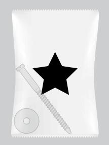
Do not discard the hardware bags or mix parts from different bags. Make note of the symbol printed on each hardware bag. The symbols can be used to identify the appropriate hardware for each step.
