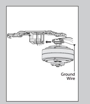
While holding the wires out of the way, lift the motor assembly and place the square hanger into the opening in the ceiling bracket. Be sure the ground wire attached to the hanger faces out of the large opening in the ceiling bracket.
