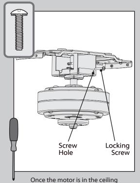
bracket, use the two locking screws found in the 🖈 hardware bag to secure the motor to the ceiling bracket.
