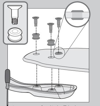
Insert grommets found in the ■ hardware bag into the holes in the blades, then secure each blade to a blade iron with screws found in the ▲ hardware bag.
