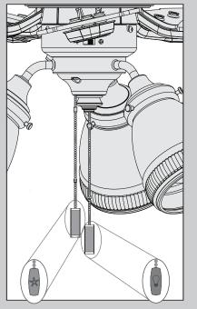
The fan pull chain controls the speed: from high to off. The light pull chain controls the light fixture: on and off.
