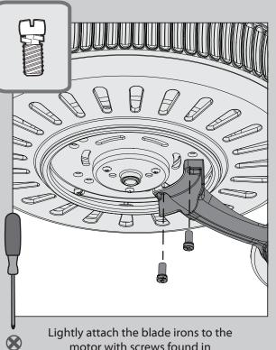
tightly attach the blade irons to the motor with screws found in the X hardware bag, then securely tighten after both screws are attached.
