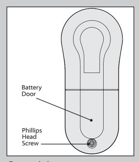
To access the battery compartment, remove the small Phillips head screw that secures the battery door to the transmitter assembly. The battery should be installed with the positive (+) side up. Replace with a CR2032 battery when necessary.
