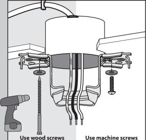
(included) when securing to support structure with approved electrical outlet box. Drill 9/64" pilot holes in support structure to aid in securing ceiling bracket with hardware found in the  $\bigstar$  hardware bag.
