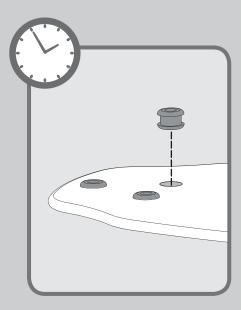
Time Saver Tip: Get a helper to insert grommets, found in the hardware bag, into the blades while you're doing the next couple of steps.
