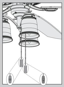
The fan pull chain controls the speed: from high to off.
