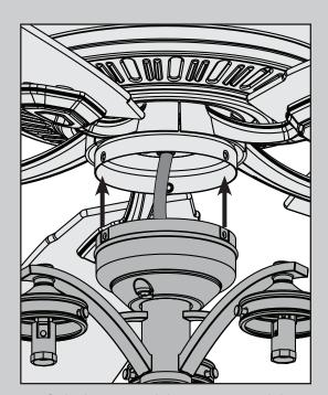
Lift the lower switch housing up until the holes line up with the screw holes in the upper switch housing.
