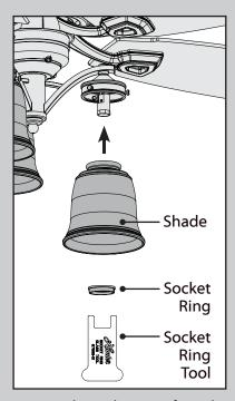
Remove the socket rings from the sockets. Install the shades onto the sockets. Install the socket rings onto the sockets. Tighten them by turning clockwise with the socket ring glass tool.
