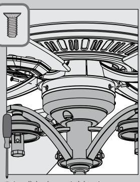
$\bigotimes$  Install the three switch housing screws, found in the  $\equiv$  hardware bag.
