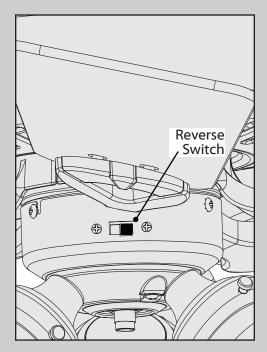
To switch the direction of air flow, move the reverse switch to the opposite position.
