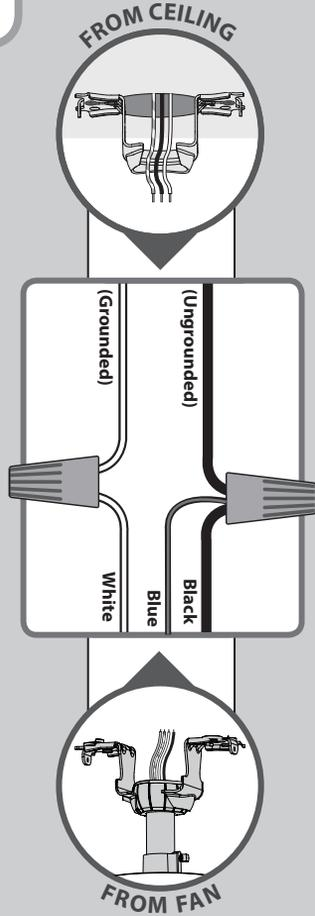
Using the orange wire connectors from the ★ hardware bag, connect the black wire (ungrounded) from the ceiling to the black and the blue wires from the fan. Connect the white wire (grounded) from the ceiling to the white wire from the fan.
