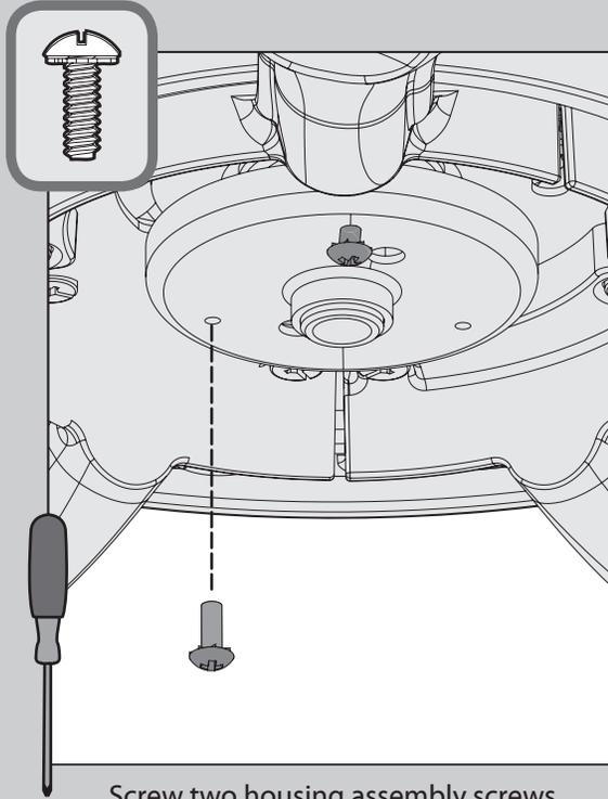
⊗ Screw two housing assembly screws from the
