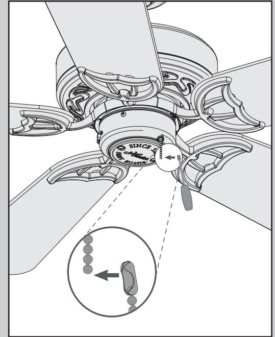
Installing the pull chain pendant - Attach the pull chain pendant to the short chain coming from the switch housing.
