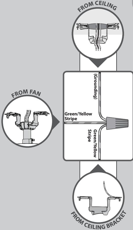
Using an orange wire connector from the ★ hardware bag, connect the 3 grounding wires (green, green/yellow stripe, or bare copper) coming from the ceiling, downrod, and hanging bracket.
