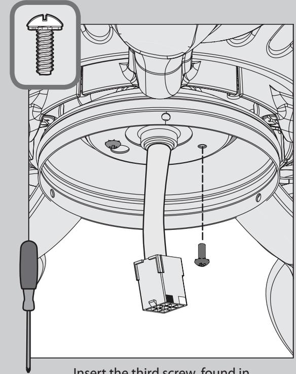
⊗ Insert the third screw, found in the
