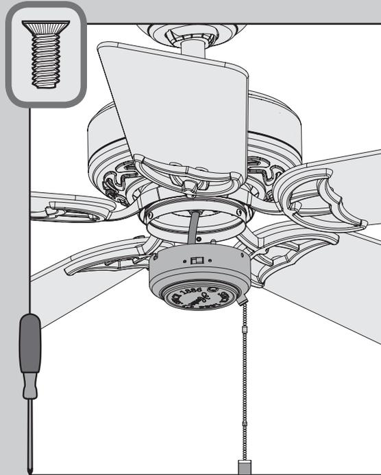
⊗ Lift the lower switch housing until its screw holes are aligned with the screw holes in the upper switch housing. Install the three switch housing screws, found in the
