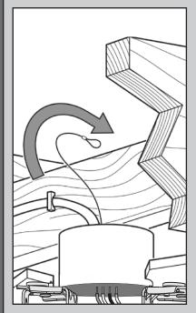
Insert the looped end of the braided cable through the ceiling bracket and one of the holes in the outlet box into the ceiling. Access the support brace in the ceiling. You may not be able to do this from below the ceiling depending on your installation site.
