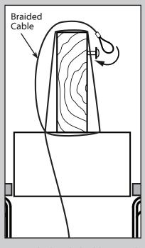
Wrap the braided cable around the support brace once creating a complete circle. Hook the looped end of the cable over the wood screw so that the cable lies between the washer and the support brace.
