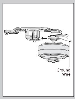
While holding the wires out of the way, lift the motor assembly and place the square hanger into the opening in the ceiling bracket. Be sure the ground wire attached to the hanger faces out of the large opening in the ceiling bracket.
