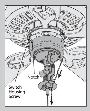
Align the notches in the sides of the lower switch housing with the upper switch housing screws. Lift the lower switch housing. Twist the lower switch housing clockwise to lock into place. Then thread the fan pull chain through the hole in the light kit.
