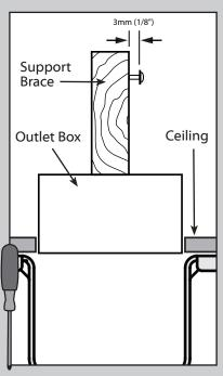
Drive the wood screw and washer found in the bag into the side of the support brace that holds the outlet box.
