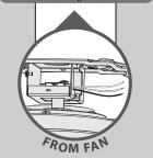
Turn the splices upward and push them carefully back through the hanger bracket into the outlet box. Spread the wires apart, with the grounded wires on one side of the outlet box and the ungrounded wires on the other side of the outlet box.
