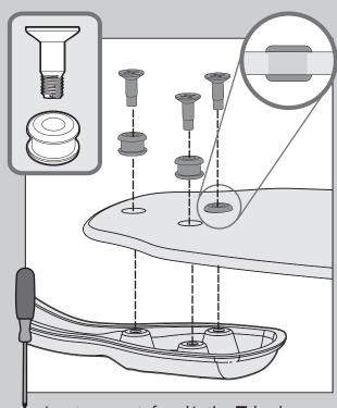
Insert grommets found in the ■ hardware bag into the holes in the blades, then secure each blade to a blade iron with screws found in the ▲ hardware bag.
