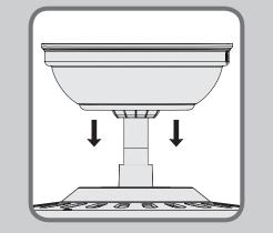
Remove the canopy. If uncertain how to remove it, reference the fan's owner's manual. With wiring exposed, it may be helpful to note existing wire connections or take a digital photo for reference. Remove the wire connectors that connect the wires from the outlet box to the fan, leaving the grounding wires connected.
