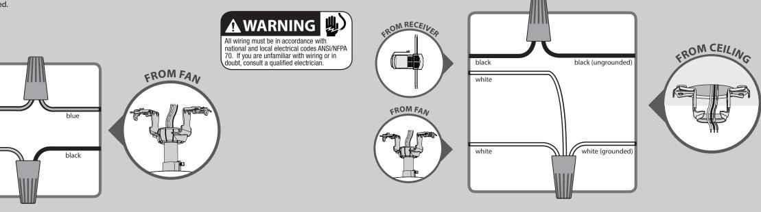
CONNECT WIRES FROM RECEIVER TO FAN - Using the orange wire connectors, connect the blue wire from the receiver to the blue wire (or possibly black with white stripe wire) from the fan. Connect the yellow wire from the receiver to the black wire from the fan.
