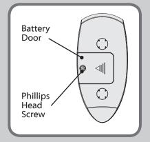
Installing or changing the battery -To access the battery compartment remove the small Phillips head screw that secures the battery door to the transmitter assembly. Replace with a CR2032 battery when necessary. The battery should be installed with the positive (+) side up.
