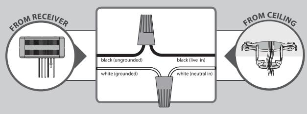
**CONNECT WIRES FROM RECEIVER TO WIRES FROM OUTLET BOX** - Using an orange wire connector connect the black wire (ungrounded) from the ceiling to the black wire from the receiver (marked "live in"). Connect the white wire (grounded) from the ceiling to the white wire from the receiver (marked "neutral in").
