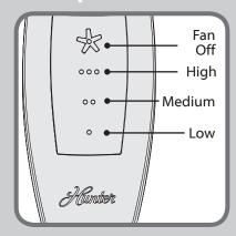
The Fan Off button only turns the fan off. To turn the fan on, press one of the fan speed buttons. They are located under the Fan Off button.
