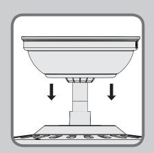
Remove the canopy. If uncertain how to remove it, reference the fan's owner's manual. With wiring exposed, it may be helpful to note existing wire connections or take a digital photo for reference. Remove the wire connectors that connect the wires from the outlet box to the fan, leaving the grounding wires connected.
