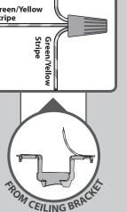
Note: To connect the wires, hold the bare metal leads together and place a wire connector over them, then twist clockwise until tight.
