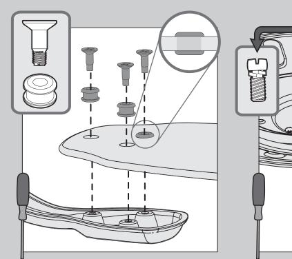
Insert grommets found in the ■ hardware bag into the holes in the blades, then secure each blade to a blade iron with screws found in the ▲ hardware bag.
