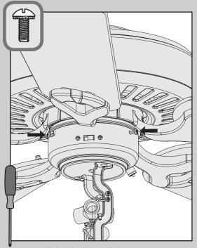
Install the third switch housing screw. Tighten all three screws securely.
