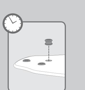
Time Saver Tip: Get a helper to insert grommets, found in the ■ hardware bag, into the blades while you're doing the next couple of steps.
