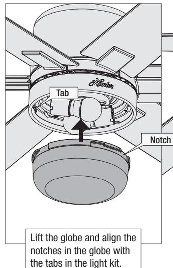
Attach the globe by lifting and turning clockwise one third of a full turn of the glass until it stops.
