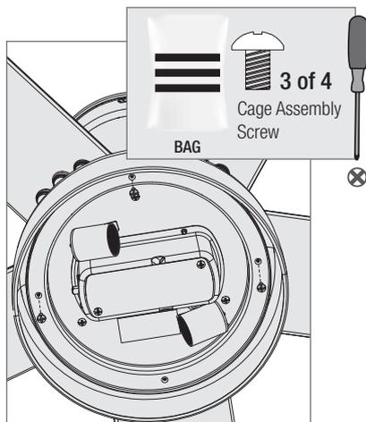
Partially install three cage assembly screws, found in the hardware bag, halfway into the light kit as shown. It does not matter which screw holes you choose.
