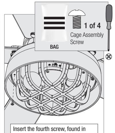
Insert the fourth screw, found in the hardware bag, in place and firmly tighten all the four screws.
