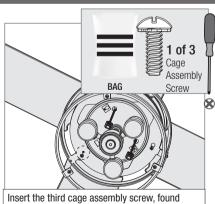
Insert the third cage assembly screw, found in the == hardware bag, in place and firmly tighten all the three screws.
