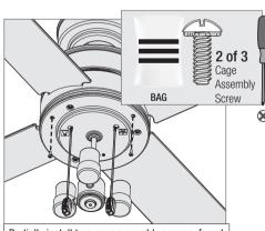
Partially install two cage assembly screws, found in the == hardware bag, halfway into the light kit as shown. It does not matter which screw holes you choose.
