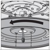
Feed the 9-pin wire plug through the center hole of the upper switch housing, then wrap keyhole slots around the screws and twist counterclockwise.
