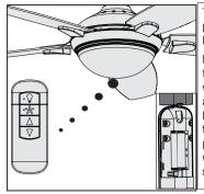
The remote transmitter is already paired to the receiver and ready to use. **Dimming mode is off by default.**
