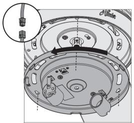
Connect the plugs from the upper and lower switch housings. Make sure to line up the colored markings on the connectors. Lift the light fixture so that the larger keyhole slots slide over the screws. Rotate the light fixture counterclockwise. Ensure all three screws are engaged in the keyhole slots.
