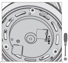
After rotating the light fixture into place, tighten all three screws securely.
