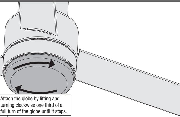
Attach the globe by lifting and turning clockwise one third of a full turn of the globe until it stops.
