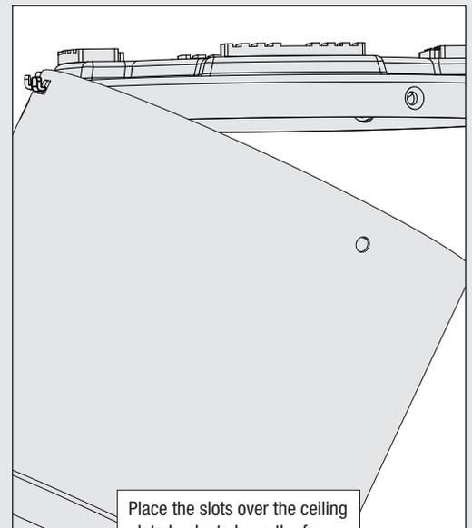
Place the slots over the ceiling plate hooks to hang the fan.
