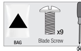
Put the blade washers found in the ■ hardware bag onto the blade screws found in the ▲ hardware bag. Then install the blade screws to secure each blade to the fan.
