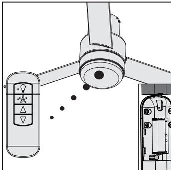
The remote transmitter is already paired to the receiver and ready to use. **Dimming mode is off by default.**
