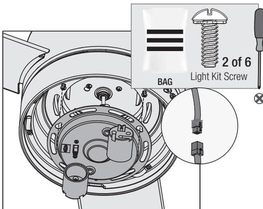
Partially install two of the light kit screws found in the hardware bag. It does not matter which two screw holes you choose. Connect the plugs from the upper and lower switch housings. Make sure to line up the colored markings on the connectors.
