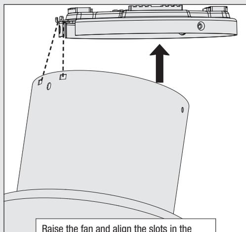
Raise the fan and align the slots in the canopy with the hooks on the ceiling plate.
