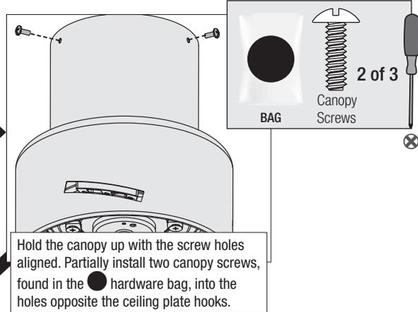
**Note:** The slots in the canopy must remain engaged while swinging the canopy for alignment.
