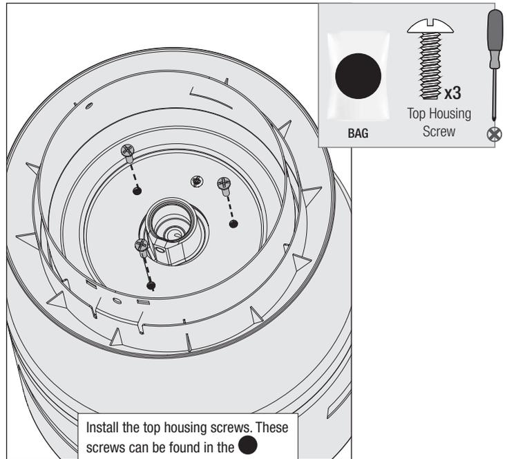
Install the top housing screws. These screws can be found in the
