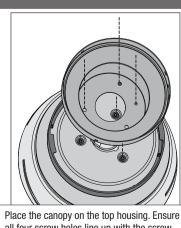
all four screw holes line up with the screw holes in both the top housing and the adapter.
