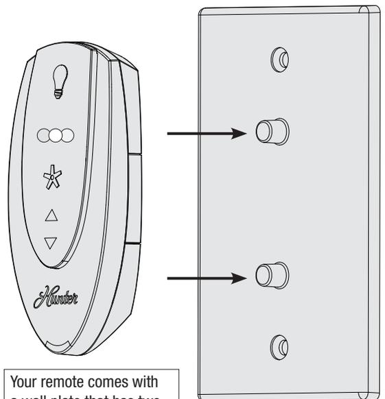
Your remote comes with a wall plate that has two posts on which to mount your remote transmitter when not in use.
