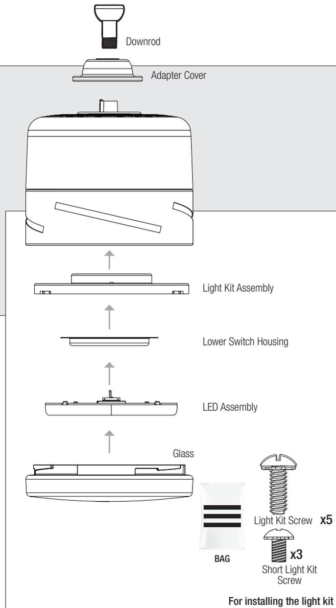
For installing the light kit
