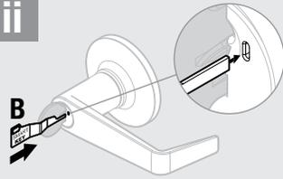
Insert SmartKey tool (B) **fully and firmly** into the hole. You may feel the tool click inside the lock.
