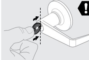
**! Make sure new key is FULLY inserted into lock.**
