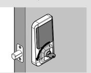
Turn the key 180° to retract the latch. Ensure that the latch retracts smoothly.
