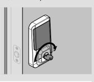
If your door does not lock and unlock smoothly, make sure you replaced your previous latch and strike with those supplied in the box. If you still experience locking errors, call Weiser Support to order a Warped Door Service Kit. Weiser Support: 1-800-501-9471
