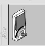
Turn the key 180° to retract the latch. Ensure that the door unlocks smoothly.
