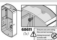
When the window is locked, you will need to remove the entire interior cover and screws to access the battery pack and buttons.
