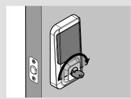
C Close the door. Insert and rotate the key to lock the door. Ensure that the door locks smoothly.
