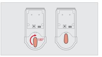
The latch is installed upside down.
