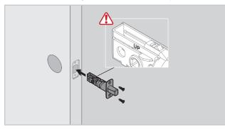
Reinstall the lock. If the turnpiece does not align with the torque blade, rotate the turnpiece 180° clockwise (you will need to use force when rotating the turnpiece, and you will hear it click).
