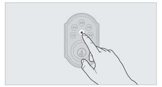
Press the Program button the number of times that corresponds to the user code position being programmed.
