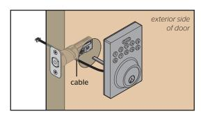
**IMPORTANT:** Make sure the latch is fully retracted (in the unlocked position).
