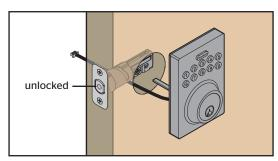
IMPORTANT: Make sure the torque blade is in the horizontal position.
