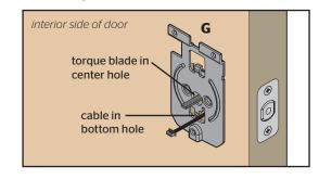
G Secure the mounting plate with the supplied screws.
