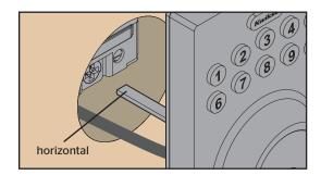
Insert the torque blade through the horizontal slot of the cross-shaped hole.
