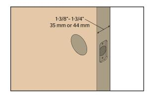
Hold the latch in front of the door hole, with the latch face flush against the door edge.
