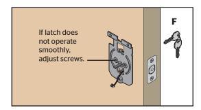
Remove the key and make sure the latch bolt is still in the unlocked position.
