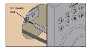
Push the torque blade through the center hole in the mounting plate and send the cable through the bottom hole.
