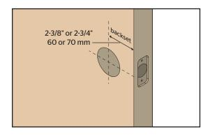
Measure to confirm that the door is either 1-3/8" or 1-3/4" (35 mm or 44 mm) thick.
