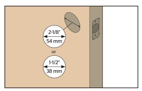
Note: Additional door preparation may be required for doors with 1-1/2" (38 mm) holes. Consult the deadbolt drilling instructions at www.kwikset.com/doorprep
