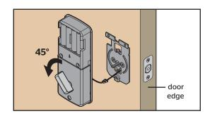
Make sure the torque blade is still in the horizontal position and install the interior assembly.
