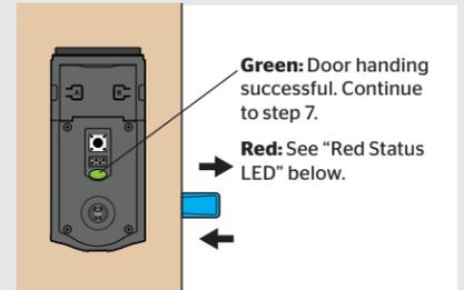
If the bolt does not move, make sure the batteries are installed correctly, and perform steps 6A-6D again.
