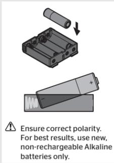
**B** Make sure the door is open. Insert the battery pack while **PRESSING AND HOLDING** the Program button. Keep pressing the button for three seconds after the battery pack is installed, then release the button.
