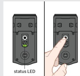
**D** The latch bolt will retract and extend on its own to learn the orientation of the door. Did the Status LED turn green or red?
