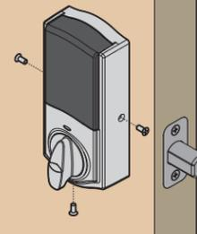
Note: The interior cover and screws must be removed for battery pack access.
