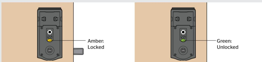
**B** If the Status LED is displaying the wrong lock status, flip switch #4.
