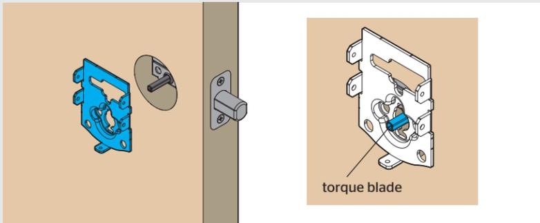
Note: A D-shaped torque blade is shown, but installation is the same for all models.
