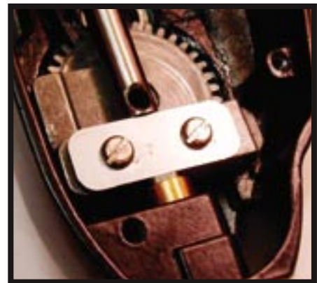
Original attachment method using two screws and a crosswind block plate
