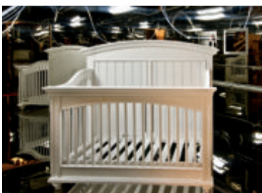
Testing in dynamic environmental chamber where air flow simulates actual use.
