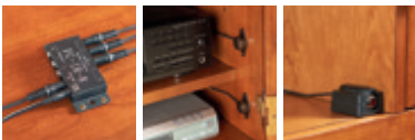
-100 INFRARED REMOTE READER The infrared remote reader transfers your remote control signals to your audio/video components even if they are positioned behind wood panel doors, eliminating the need to insert glass panels. The infrared reader includes a receiver with mounting block, an infrared repeater control unit with power cord and three emitters. Each emitter, when properly positioned on the interior of the case, will transfer your remote control signal to the audio/video components positioned on one shelf. The system is easy to install and use. No programming is needed and the emitters may be repositioned as your audio/video components or configurations change.
