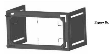
• Gently tighten the Connector Bolts in a Clockwise motion with the Allen Wrench provided. Do not completely tighten at this time. See Figure 3c.
