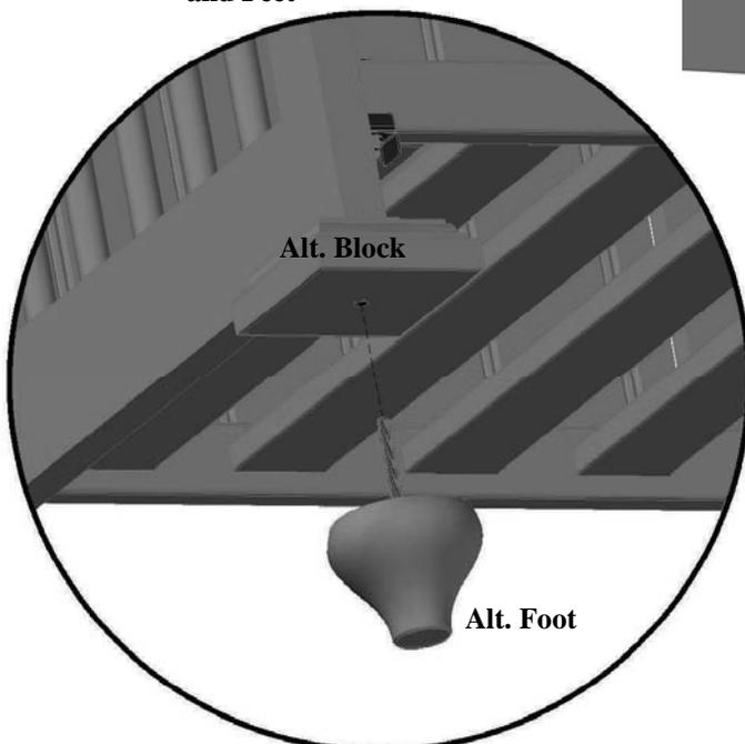
Fig. 16 Attaching Alternate Foot
