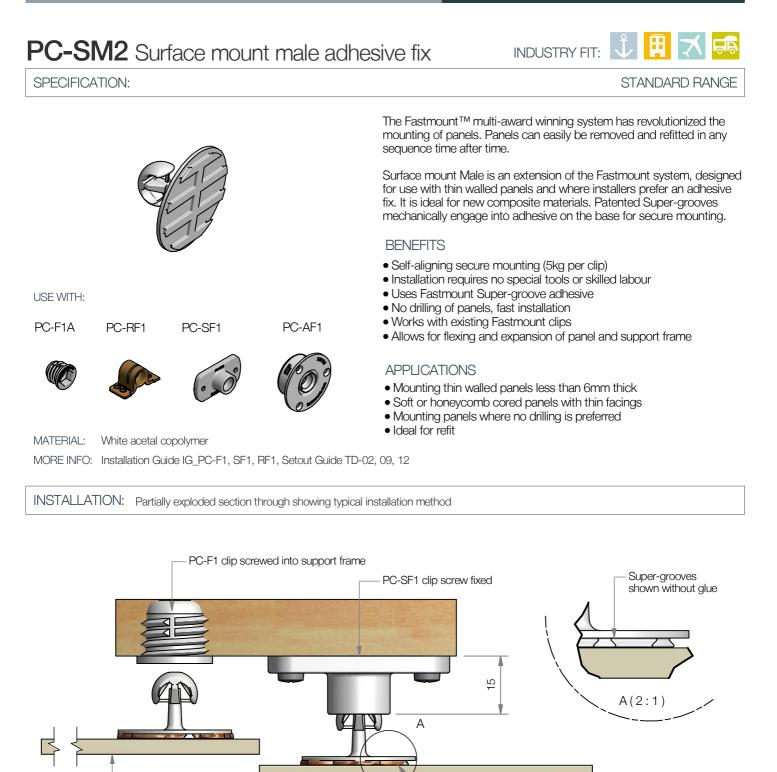
FM Super-groove adhesive applied to PC-SM2 flows around super-grooves
