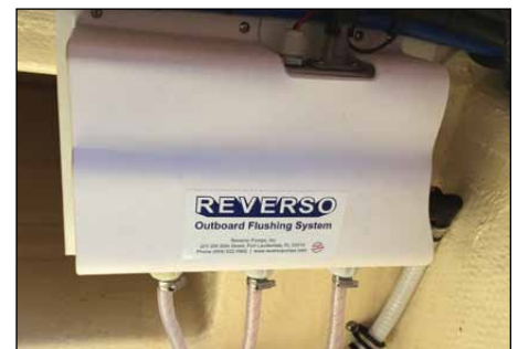
Mounted inside hull compartment
