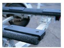
E-Z Slide Bunk Enders work with 4" or 6" bunks. Mount them towards the inside edge of the bunk where initial contact and heavy wear are most common.
