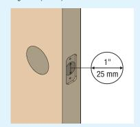
Measure to confirm that the door is either D 1-3/8" or 1-3/4" (35 mm or 44 mm) thick.
