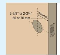
Measure to confirm that the hole in the door edge is 1" (25 mm).
