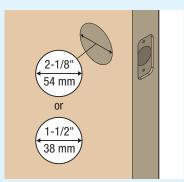
Note: Additional door preparation may be required for doors with 1-1/2" (38 mm) holes. Consult the deadbolt drilling instructions at www.kwikset.com/doorprep.
