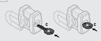
Close shackle. The key will automatically rotate back to the home position. The lock has been successfully re-keyed.
