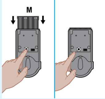
**C** The Status LED will flash red and green, and the lock will beep. Press and release the Program button again. The latch bolt will retract and extend on its own.
