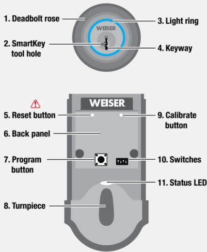
1. Touch Kevo anywhere on the metallic surface behind the light ring to lock and unlock.
