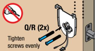
**e** Insert key and test latch. If latch does not extend or retract smoothly, adjust screws (Q/R). Remove key when finished and make sure the latch bolt is fully extended.
