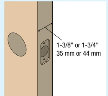
Note: Additional door preparation may be required for doors with 1-1/2" (38 mm) holes. Consult the deadbolt drilling instructions at [www.weiserlock.com/doorprep](http://www.weiserlock.com/doorprep).
