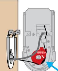
**c** Lay thicker cable flat against the interior housing.
