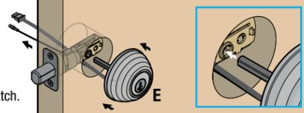
**c** Route cables through center hole, then push cables into side hole.
