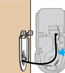
**d** Push the turnpiece shaft onto the torque blade. Avoid pinching the excess thinner cable by pulling it away from the torque blade.
