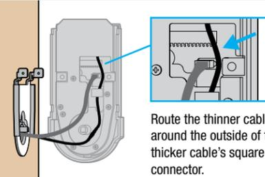
**b** Tuck the thinner cable's connector behind the backplate (as indicated by the sticker on the interior assembly).
