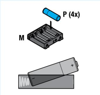
⚠ Ensure correct polarity. For best results, use new, non-rechargeable Alkaline batteries only.
