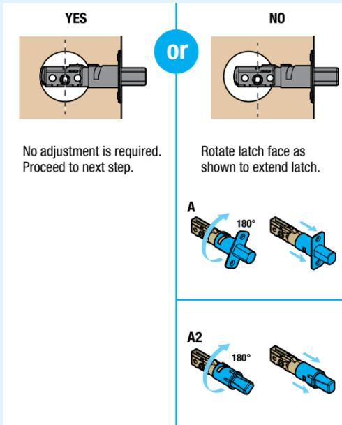
**D** Which latch are you installing?
