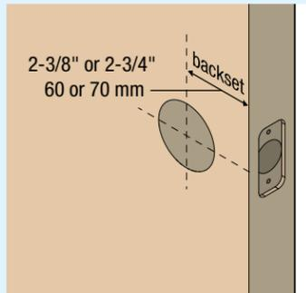
**C** Measure to confirm that the hole in the door edge is 1" (25 mm).
